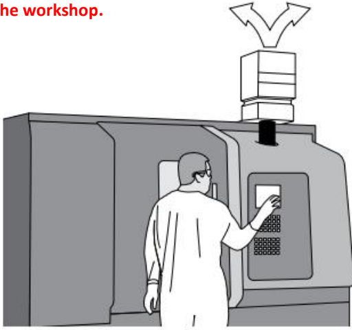
CNC machine with a standalone LEV fitted
